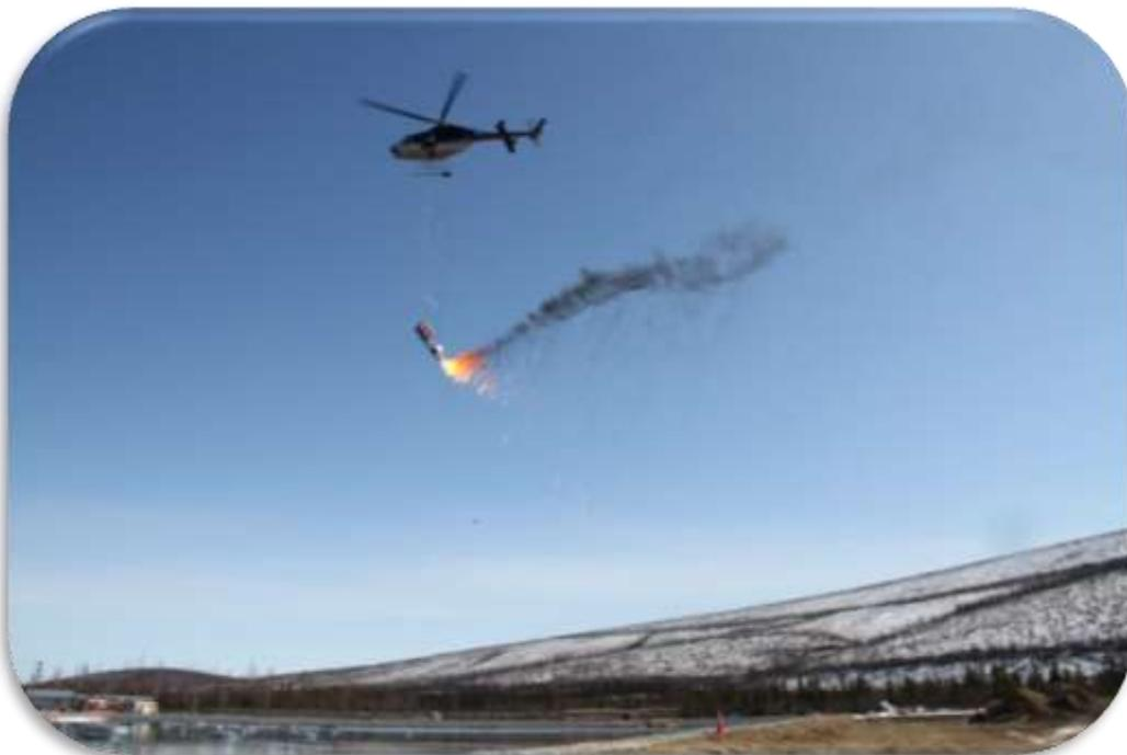
Using a heli-torch to light oil in a test basin. Picture from <http://arcticresponse.wpengine.com/wp-content/uploads/2017/09/poker-flats-report-final.pdf>.
