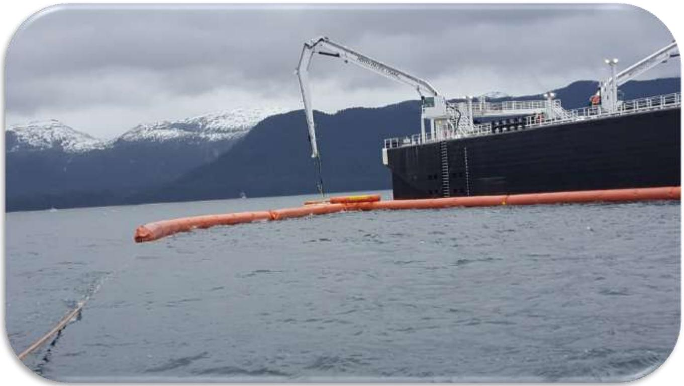
Practicing with the new open water barge in Prince William Sound. A new series of barges were introduced to Prince William Sound in 2018. These barges use new boom and skimmer designs to improve response speed and efficiency.
