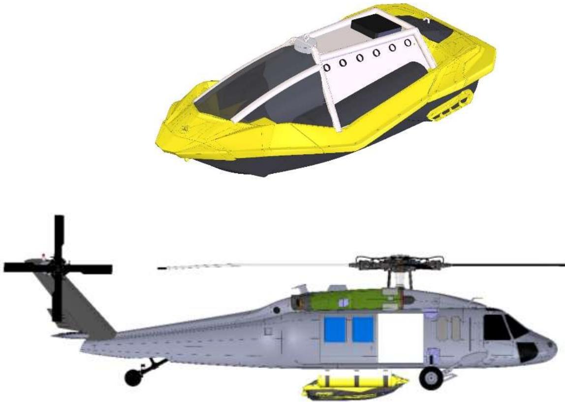
Based on the initial work sponsored by OSRI, the Herder/Ignitor Joint Industry Program decided to move forward with the development of an unmanned surface vessel that can be winched up under a helicopter for delivery of chemical herders and ignition. We will also be developing a new ignition system that can be carried in the helicopter to use with the existing chemical herder deployment system.
