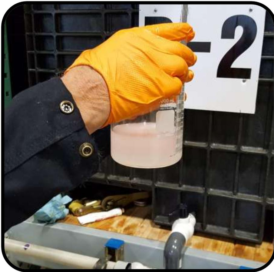
Examining recovered diesel oil for water during skimmer efficiency testing.
