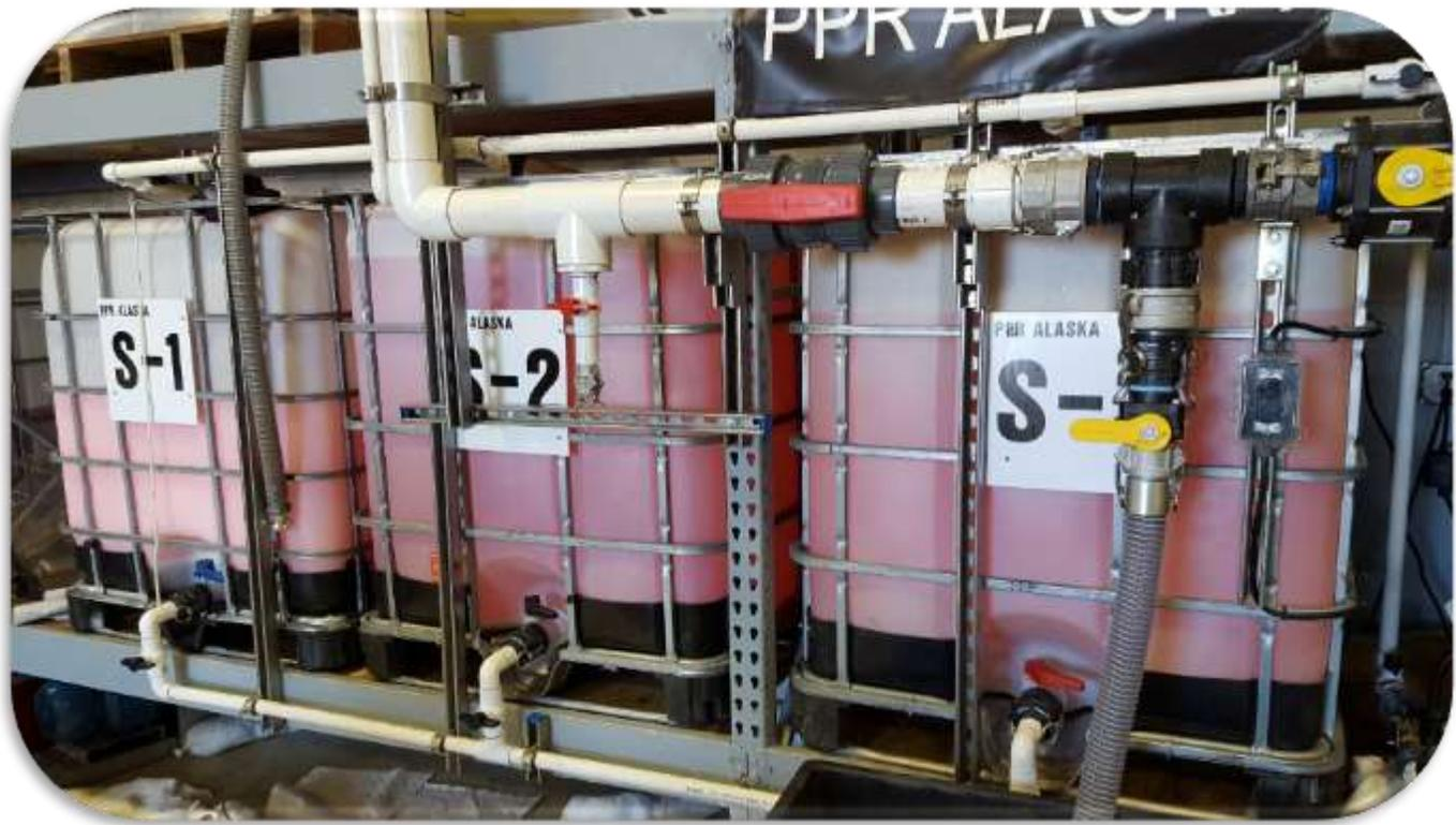
Colored diesel oil was used to test the efficiency of oleophilic skimmers.
