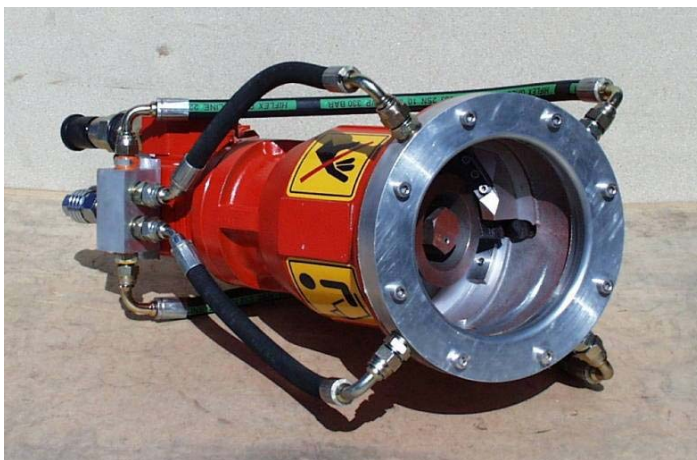
Figure 2 DOP-160 with flemingCo inlet side steam/hot water injection AWIF
